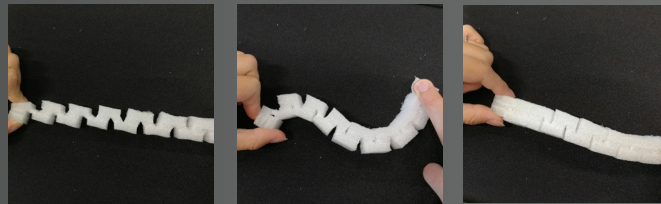
Fig 7. Three different movements of foam with cuts (bended, pushed, pulled)
