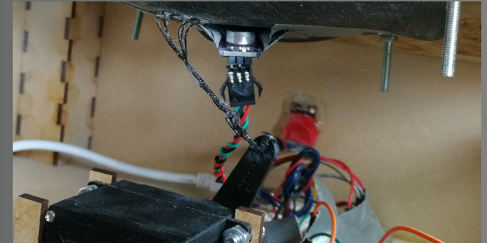
Fig 14. Inside of the box where the servo and internal microphone are attached to material
